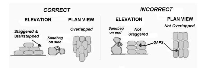
Figure 4 – Correct and incorrect placement of staggered sandbag layers.
