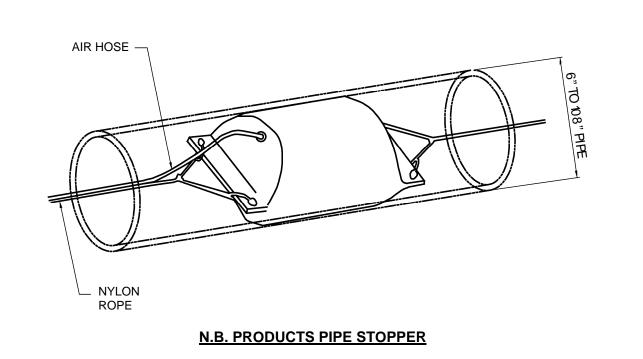
N.B. PRODUCTS, INC. MANUFACTURES A RUBBERIZED PIPE STOPPER IN ALL STANDARD PIPE SIZES FROM 6" TO 108". THE COST FOR THESE DEVICES RANGES FROM \$20.00 TO \$3,000.00 ADDITIONAL EQUIPMENT REQUIRED FOR INSTALLING THE PIPE STOPPER ARE AN AIR HOSE KIT, AIR HOSE, AND NYLON ROPE. A TWO-WEEK SHIPPING PERIOD IS REQUIRED. MANUFACTURING LEAD TIME IS REQUIRED FOR SIZES OVER 60". ORDERS FOR THESE UNITS CAN BE PLACED TO:
