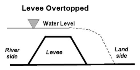
Breach - Does not imply cause of breach is known; However, the levee has been compromised by overtopping, and repairs are necessary.
