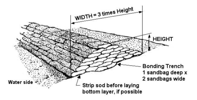
Figure 2 – Proportions of sandbag dike showing bonding trench at base.
