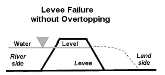
Failure without Overtopping - Implies the cause of breach is known to be a result of poor levee performance and occurred without overtopping. This designation should only be applied where studies and investigations have revealed the cause of the breach with little uncertainty.
