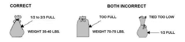
**Figure 1 – Correct and incorrect sandbag preparation.**
