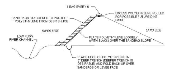
Figure 7 – Poly anchored within a trench – placed under dry conditions.
